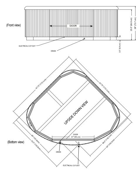
**NOTE:** Watkins Manufacturing Corporation recommends that the TX be installed on a minimum 4" (10.2cm) thick reinforced concrete pad or structurally sound deck able to support the "dead weight" found in the spa specification chart.
