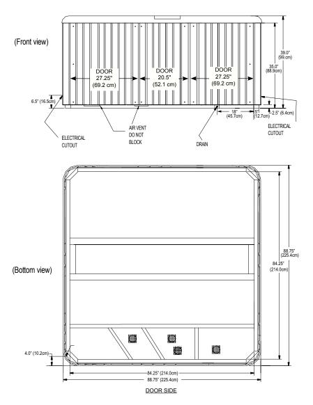
**NOTE:** Watkins Manufacturing Corporation recommends that the Tempo be installed on a minimum 4" (10.2cm) thick reinforced concrete pad or structurally sound deck able to support the "dead weight" found in the spa specification chart.
