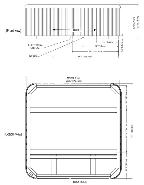
**NOTE:** Watkins Manufacturing Corporation recommends that the SX be installed on a minimum 4" (10.2cm) thick reinforced concrete pad or structurally sound deck able to support the "dead weight" found in the spa specification chart.
