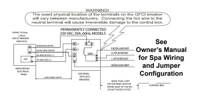
field wiring access panel of the control box. A licensed electrician should install a four-wire electrical service (two line voltages, one neutral, one ground) from the main electrical service panel to the subpanel.
